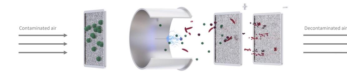
The Potok technology is used to decontaminate air by exposing microbial cells or viruses' secondary and tertiary structure of proteins to constant electric fields of a given orientation and tension. The value of the electric field is designed to destroy (not just filtrate) any microorganisms and viruses, regardless of the type (incl. mold and yeast)
